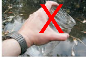
DO NOT touch openings of bottles. Keep bottles clean to prevent contamination.
