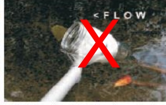
DO NOT sample with the bottle opening facing downstream, when using a pole or sampling by hand. Water flowing past your container, pole, or hand and into the container can be contaminated by such contact.
