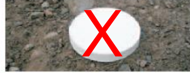
DO NOT allow bottle lids to touch ground. Keep lids clean to prevent contamination.
